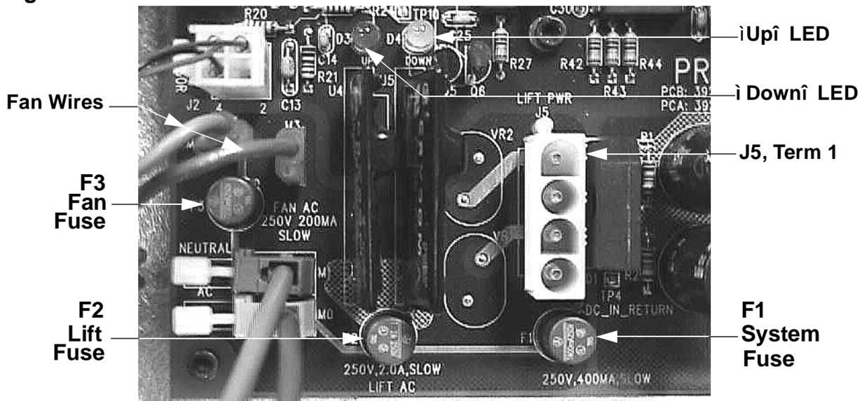
4. Insert the treadmill's line in the AC outlet and set the circuit breaker in the **on** position. Set the treadmill in the manual program and press the **LIFT ▲** key. If the lift motor operates normally, test treadmill operation per Section 3. If the lift motor still does not operate, retest the lift fuse per steps 2 & 3. If the fuse is open again, continue with step 13. If the fuse is good continue with step 5.
